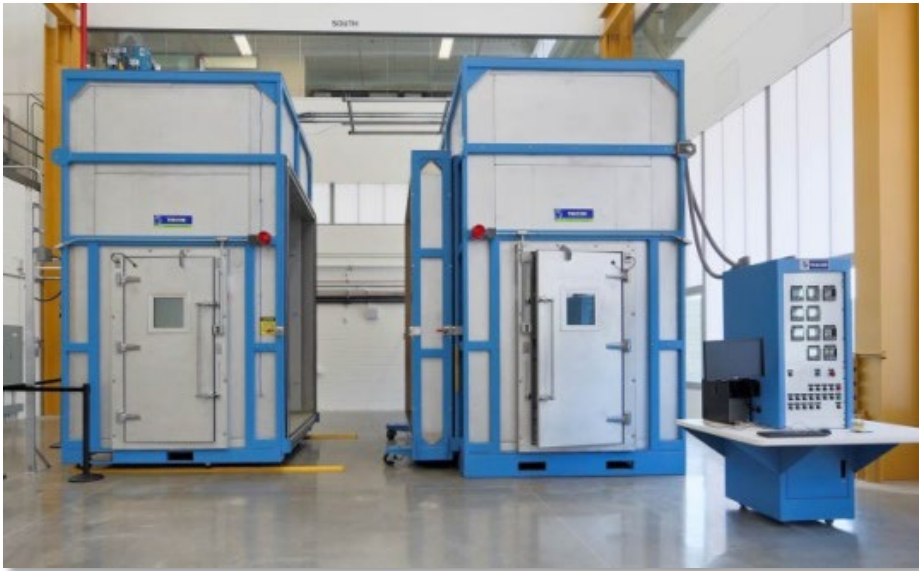
Physical thermal “hot box” testing Oak Ridge National Laboratory
