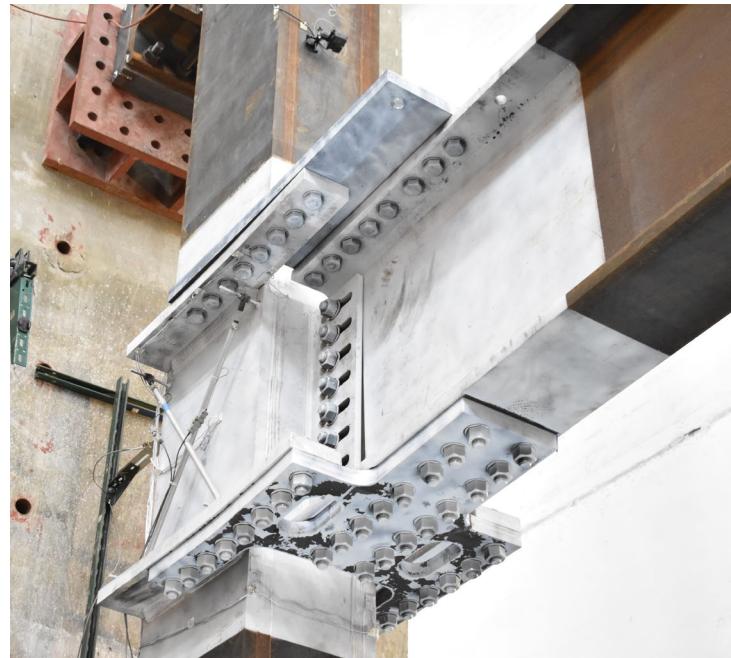
Steel Moment Connection with Bottom Flange Fuse Plate (2022)
